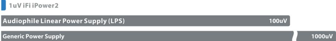
\*Noise floor is the random noise and excl. AC mains related components and switching freq (<30uV).
